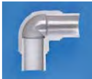
Socket fusion joining is primarily used for efficient pre-assembly in the workshop.
